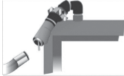
45 degree hose port pull-away: 1,300 lbs. of pull force
