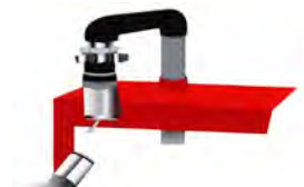
90 degree hose port pull-away: 900 lbs. of pull force
