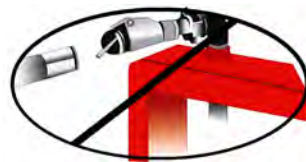
Horizontal or straight line hose port pull-away: 8,900 lbs. of pull force
